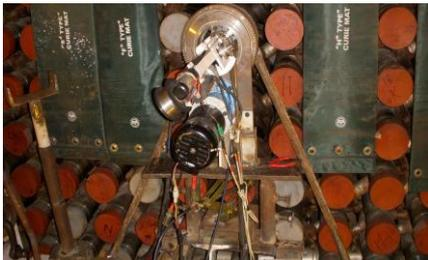
A light-water leak in O-10 channel of tri-junction weld joint between the calandria-side tube sheet, baffle plate and the lattice tube was detected and successfully repaired in Kaiga-3 south end-shield. The biggest challenge was to restrict the temperature of the nearby calandria tube rolling joint, which was only 2-3 mm away from the repair spot. Utmost care was exercised to avoid any damage to this rolled joint due to tools or heat input.
