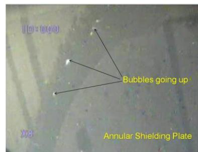
A half-scale mock-up of CV was designed and constructed. End-shield support plate and dry pack areas were simulated in the concrete wall of the mock-up. Artificial defects were created in the mock-up to simulate the defects in the liner.
